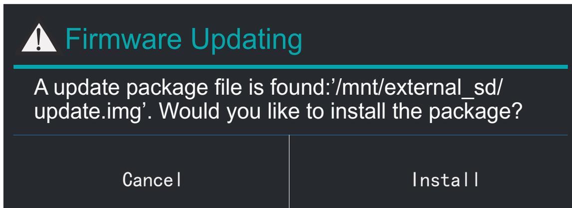
4. Choose "Install" , and Airlinker system will run update.img. Meanwhile, system will reboot, then a green robot and progress bar will be shown on the screen, until the system reboot and return to standby interface, the update process is successful.
